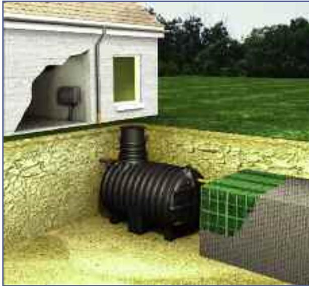
Rainwater harvesting systems can also be used to reduce stormwater run-off rates. (Picture credit: Hydro International)
