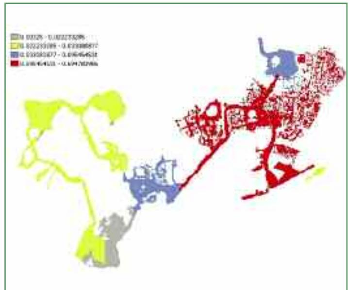
Figure 3: Average maximum velocity the two-dimensional shallow water equation modelling package TUFLOW.
