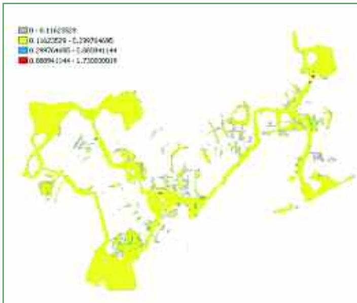
Figure 2: Final water depth using Heriot Watt's Rapid Flood Inundation Model.
