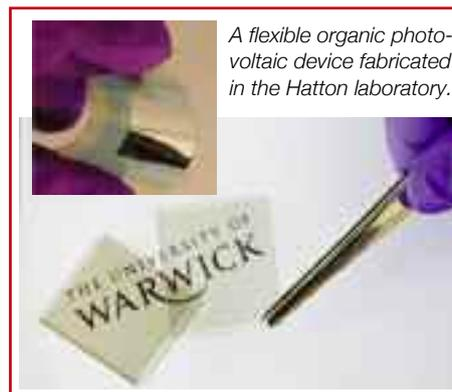
*A flexible organic photovoltaic device fabricated in the Hatton laboratory.*
