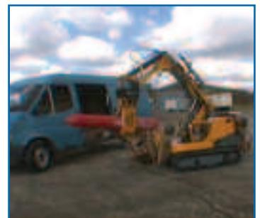
Photo 1 – An ROV gains access before searching and identifying types, sizes and ownership of the cylinders inside.
