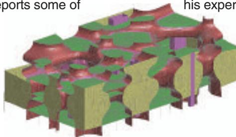
*Finite Element Model of an Opera House*
