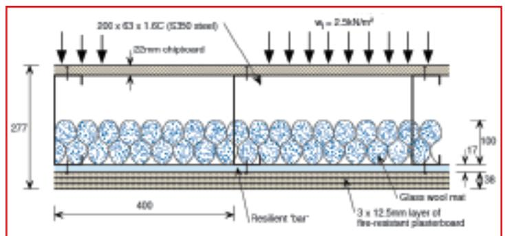
(Above) Cross section through the light steel test floor for 90 minutes fire resistance
