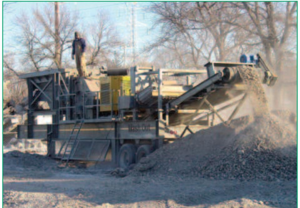
*The crushing of concrete demolition waste greatly increases its surface area and the subsequent uptake of CO<sub>2</sub>*
