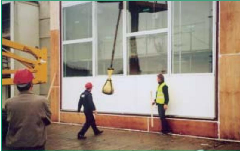
Impact testing of a curtain wall
