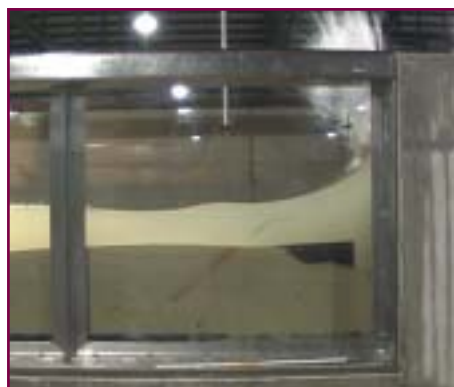
Examining the impact of storm waves on toe scour in front of a vertical sea-wall in one of HR Wallingford's wave-flumes.
