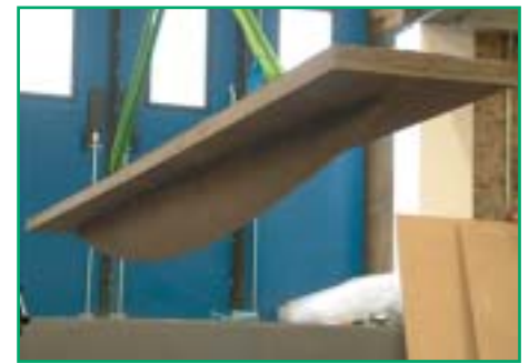
(Right) Example of a beam produced using fabric formwork.
