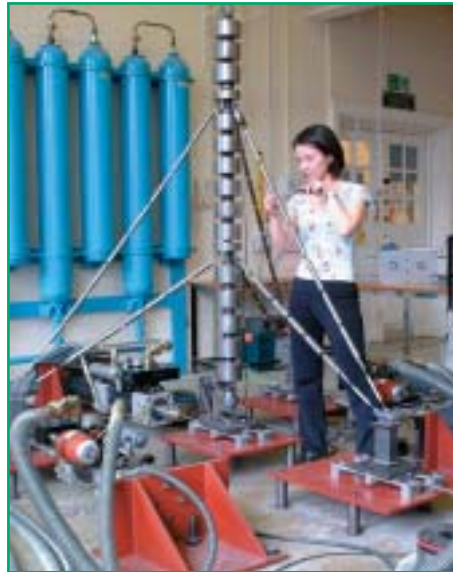
(Above) Real time hybrid test on a Jarret damper in the Structural Dynamics Laboratory at Oxford (Above right) Pseudodynamic test of a 'zipper' frame in the NEES laboratory at University of California at Berkeley
