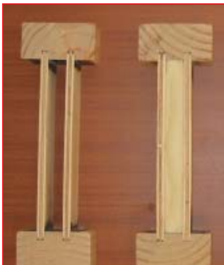
(Top): Mr Ali Bahadori Jahromi at the New Zealand Forest Research Institute. (Above): CIB Cross Sections Tested
