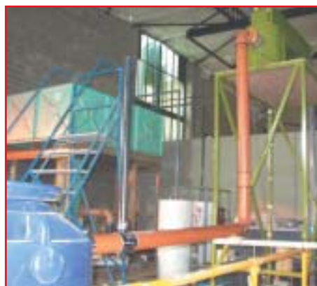
HR Wallingford's experimental hall: Rig used to develop the proposed new standard test for grease separators
