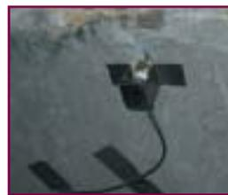
Small, discrete sensors 'listening' for corrosion activity
