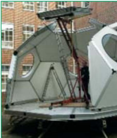
RPJS in open position with section of composite panel
