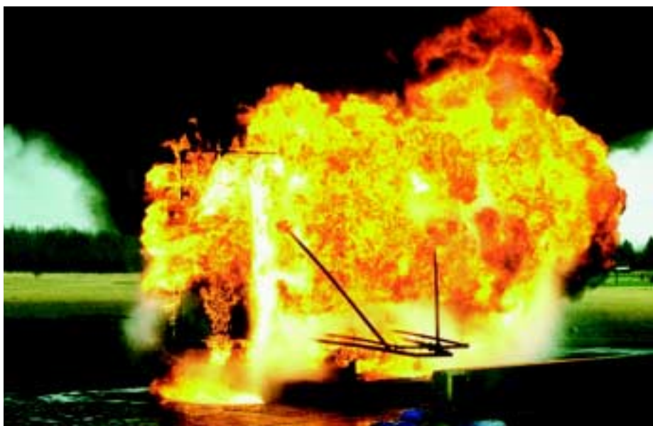
Results from hydrocarbon fire tests are used to generate typical heat-flux values to be used in estimating fire loading and response of offshore structures
