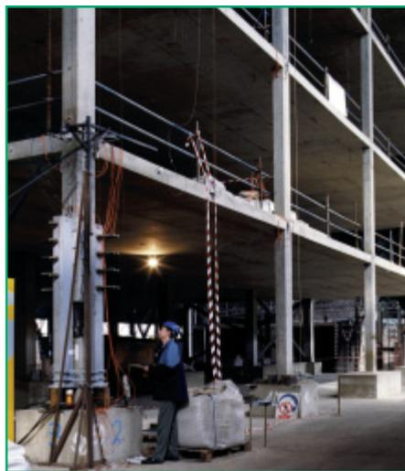
A section from the ground floor corner column of a seven-storey building has been removed to test the building's robustness.
