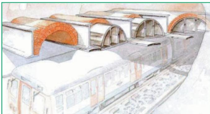
Schematic of CFRP roof strengthening
