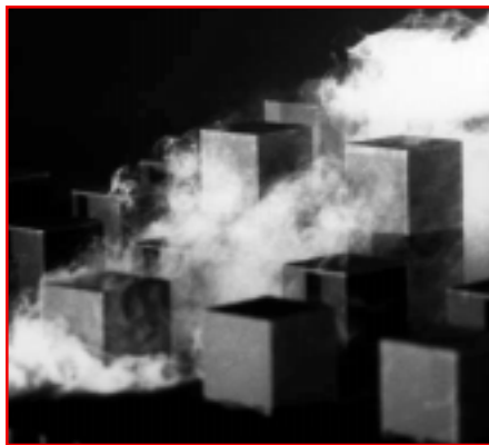
Wind tunnel studies of the dispersion of pollutants from a point source around tall buildings
