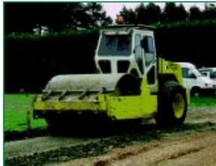
Full-scale trial of a vibrating roller on TRL vibration test pad
