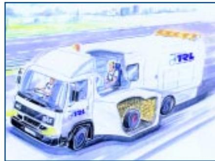
New test vehicle for tyre noise testing
