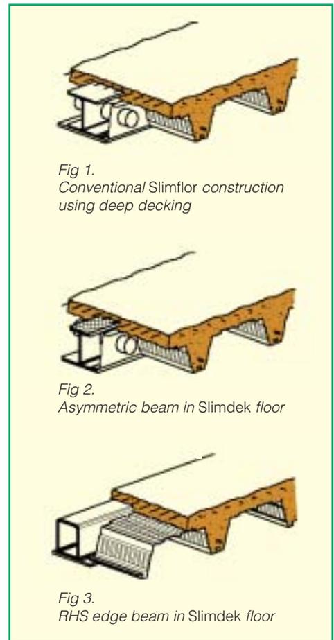
Fig 1. Conventional Slimflor construction using deep decking
