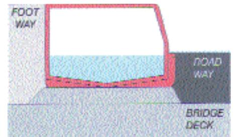
*Cross-section of a typical combined kerb drainage unit.*
